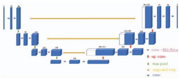
Figure 2. Structure of 3DU-Net
