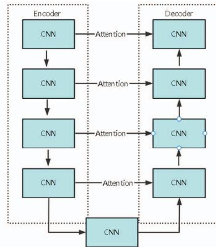
Figure 3. The architecture of Multi-Res-Attention UNet
