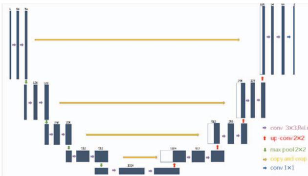
Figure 1. Structure of U-Net
