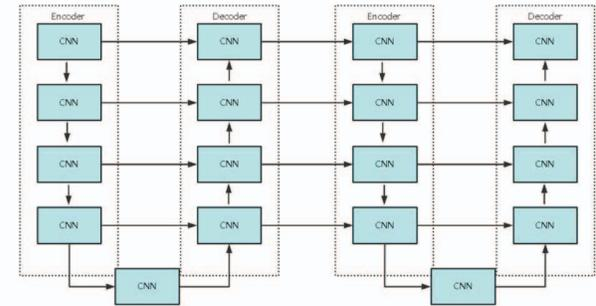
Figure 12 . The architecture of Connected-UNets
