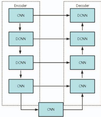
Figure 4 . The architecture of DUNet
