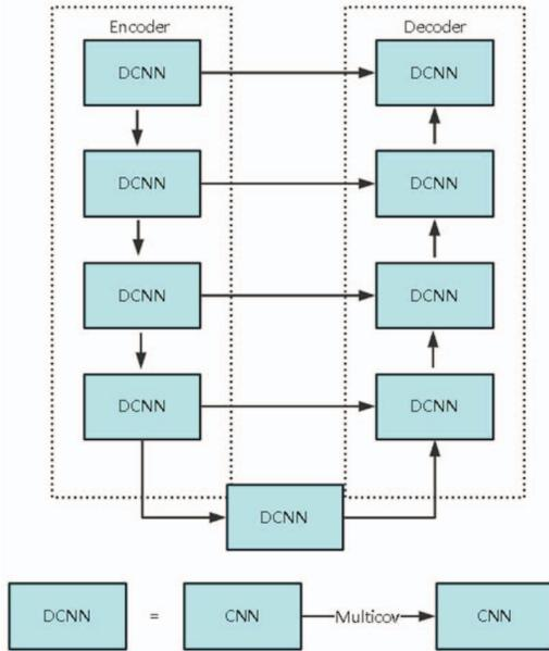
Figure 5 . The architecture of MRUNet
