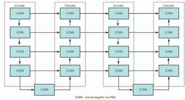
Figure 11 . The architecture of LadderNet
