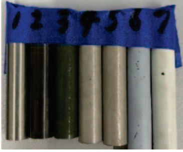
Figure 3. ZrO 2 coated rod samples: the ones labeled 1,2,3,4,5 are 0 um, 5 um, 15 um, 30 um, 45 um thick and coated with process-1 and the ones labeled 6,7 are 30 um, 45 um thick and coated with coating process-2
